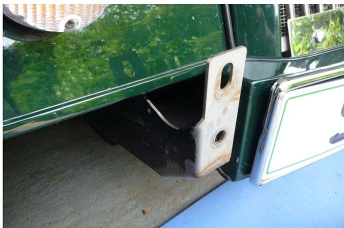
The original mounting hole (slot) is on the top and the new hole is 50mm lower. It was not that simple but a good drill with a sharp bit (and file) did the job on this strong alloy
