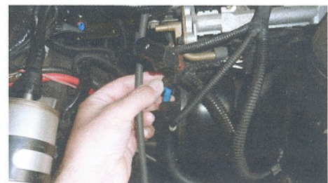
Remove loom clip to allow movement of loom
