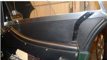
fitting it to the windscreen bracket I reversed it and fixed it to the inside channel of the side screen. This means that the 'U' channel faces the direction of the air pressure and so keeps an effective seal at speed. The channel also acts as a 'gutter' and channels water from the roof and windscreen 'down' rather than 'in'!
